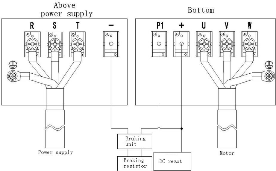
Fig 2-7 3160G/3185P~3355G/3400P Main Circuit Wiring
