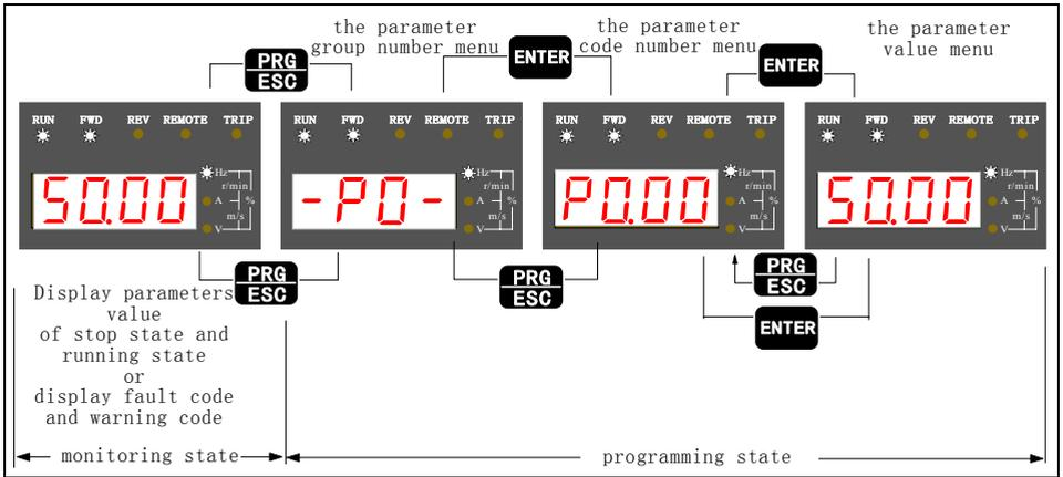
Figure 3-4 Display menus of programming state
