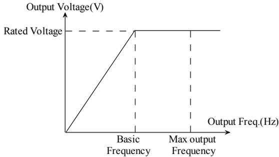
Fig. 5-0-1 V/F characteristic diagram
