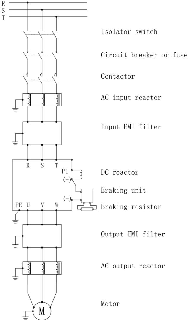
7-1 S2R4GB~3015GB/3018PB Diagrams of Peripheral Equipments
