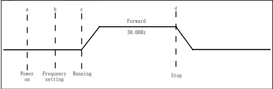
Figure 3-13 Sequence of terminal operation
