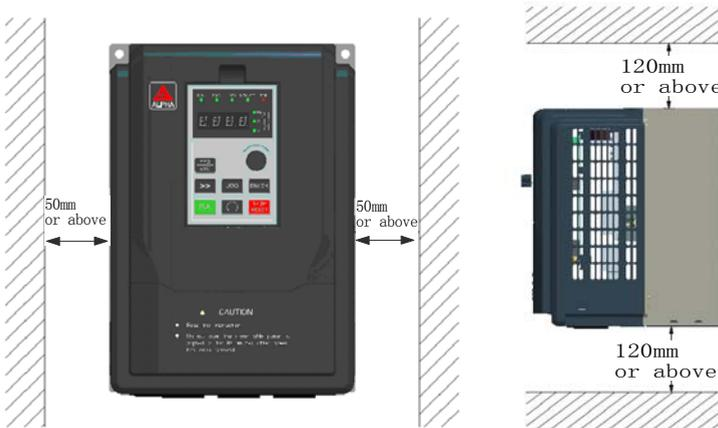
Fig 2-1 Installation Direction and Space
