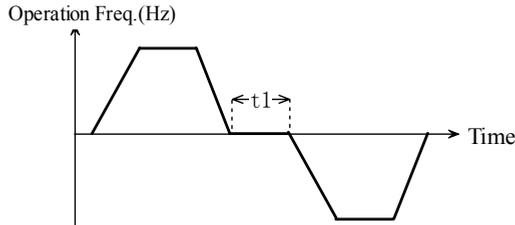
Fig. 5-2-2 FWD/REV switching time diagram
