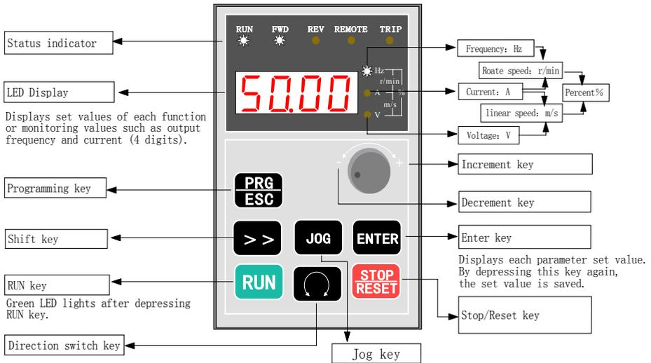
Figure 3-1 Layout and function of Keyboard
