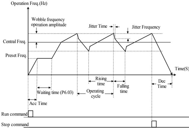
Fig. 5-6-1 Wobble frequency operation diagram
