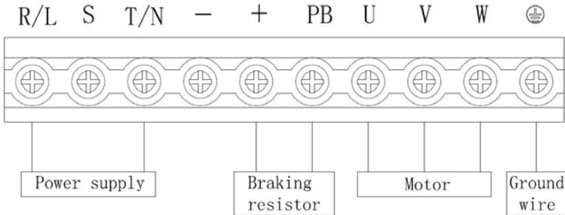
Fig 2-3 S21R5GB~S22R2GB Main Circuit Wiring
