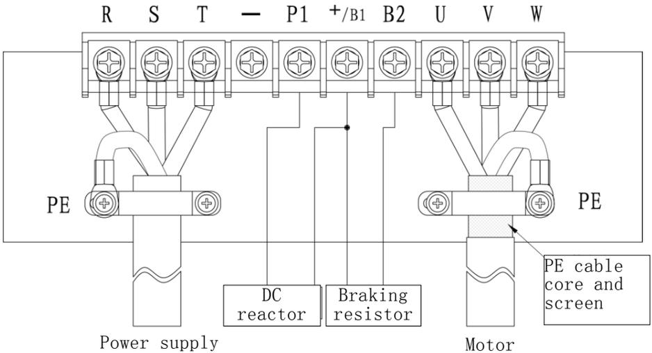
Fig 2-5 35R5GB/37R5PB~3015GB/3018PB Main Circuit Wiring
