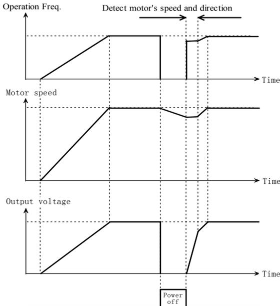
Fig. 5-1-2 Speed tracking restart diagram
