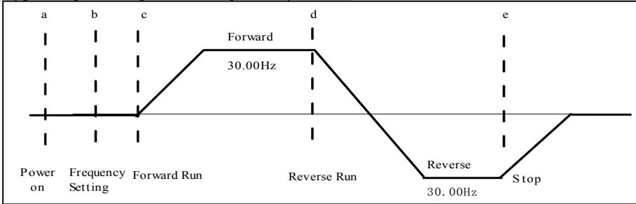
Figure 3-10 Operation sequence by keyboard
