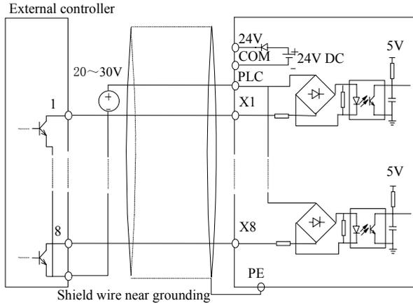
Fig 2-23 Source Connection Method
