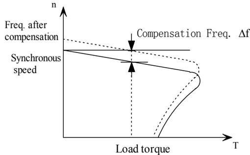
Fig. 5-9-1 Auto slip compensation diagram
