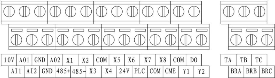
Fig 2-12 35R5GB/37R5PB~3500GB Arrangement of Control Circuit Terminals
