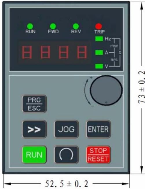
Fig. A5-1 Keyboard Mounting Size of S2R4GB~3004GB
