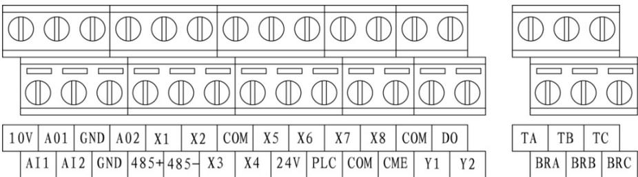
Fig 2-11 S2R4GB~3004GB Arrangement of Control Circuit Terminals
