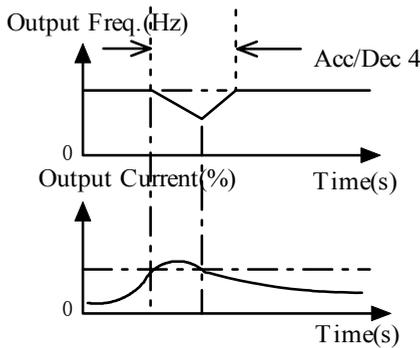
Fig. 5-13-4 constant speed Operation
