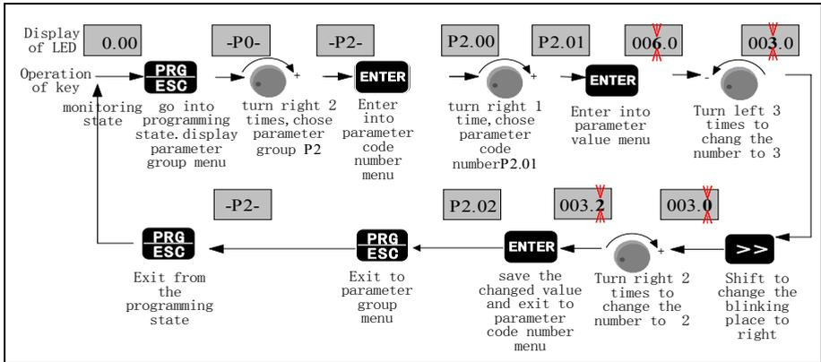
Figure 3-7 Flow chart of parameter setting
