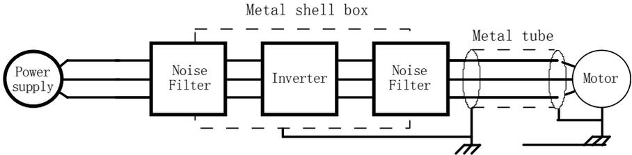
Fig 2-10 Method to Restrain RFI
