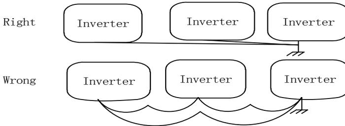
Fig 2-9 Earthing Connection Method
