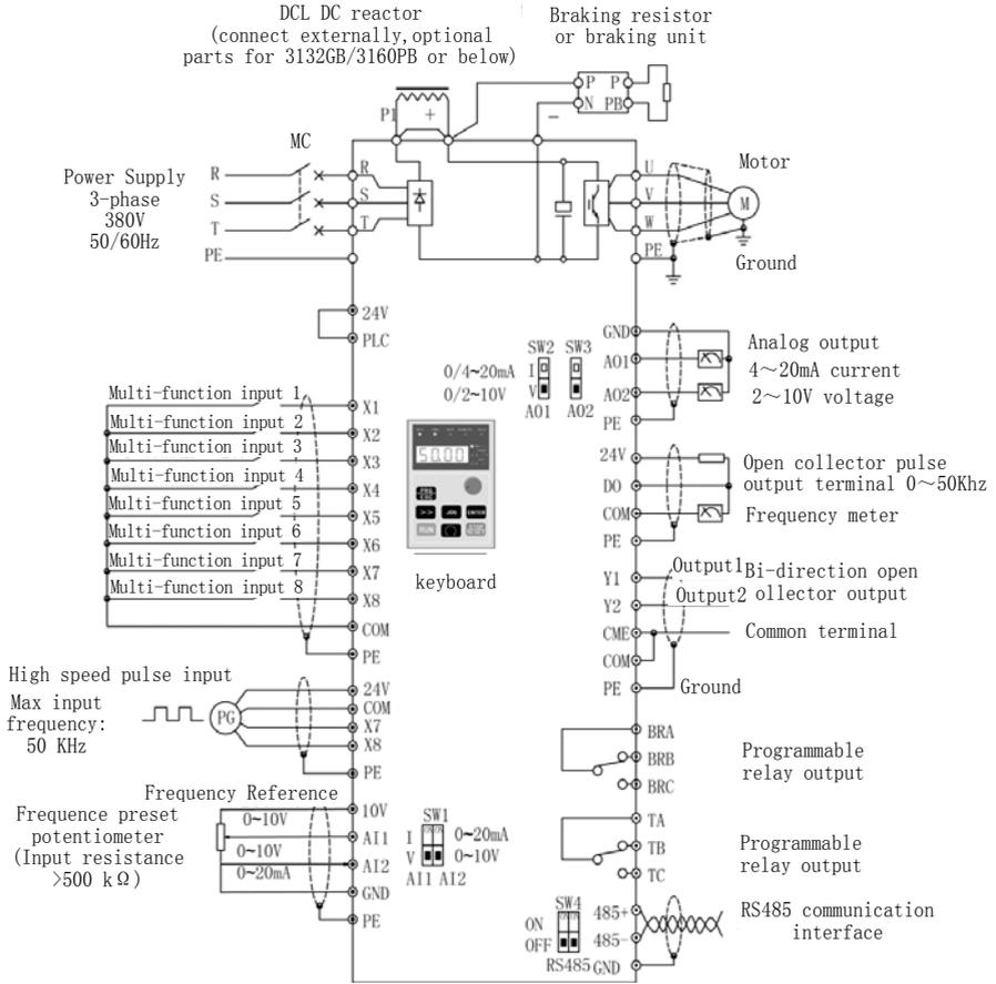
Fig 2-35 3018G/3022P~3500G Wiring diagram
