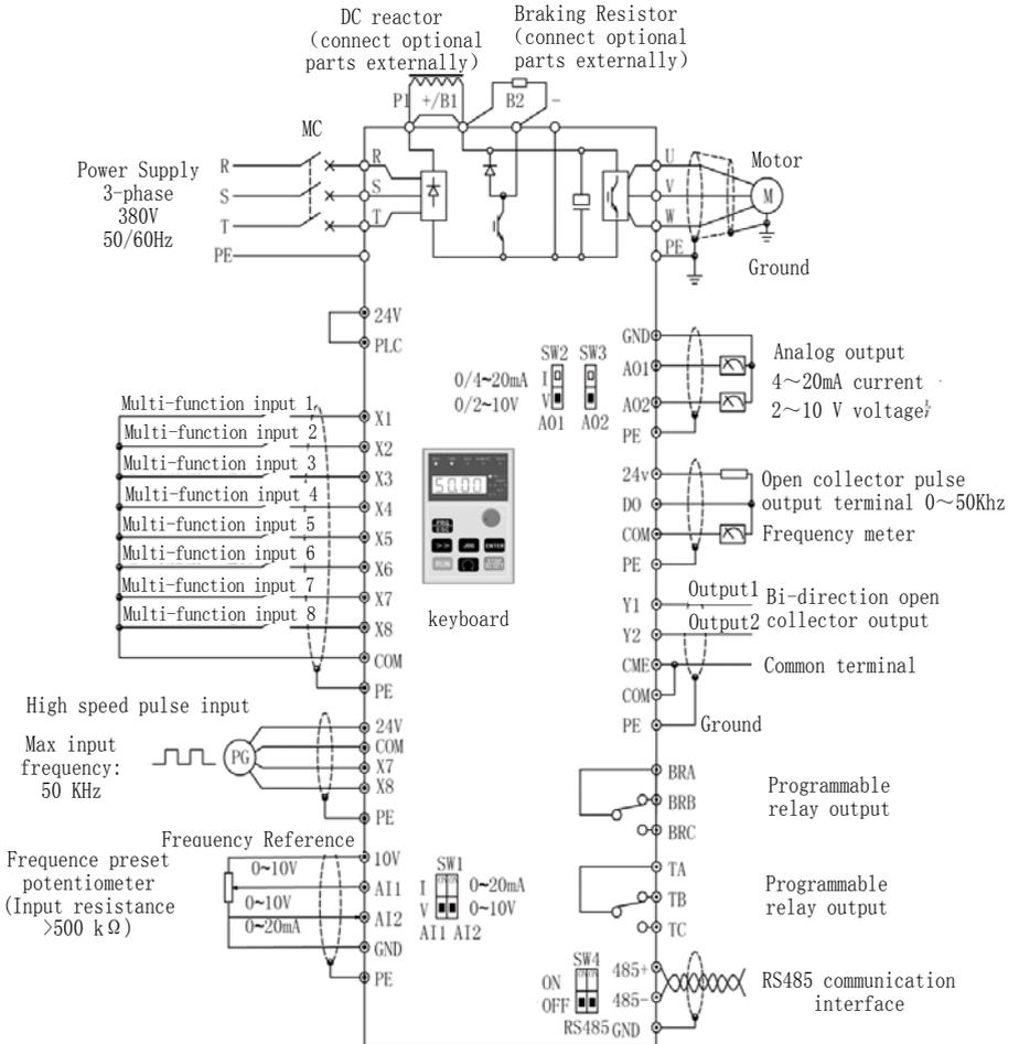
Fig 2-34 35R5GB/37R5PB~3015GB/3018PB Wiring diagram
