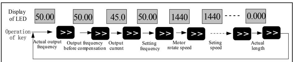
Figure 3-5 Flow chart of monitoring object switching
