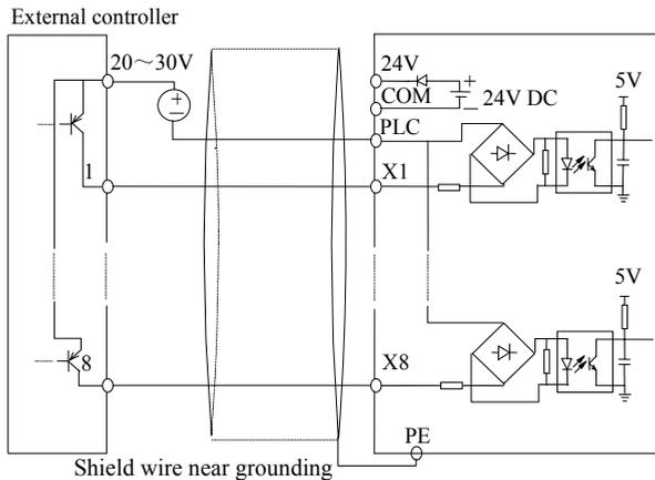
Fig 2-24 Drain Connection Method(in S2R4GB~3004GB only X1~X5)
