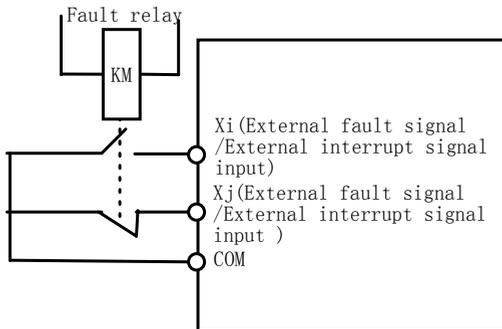
Fig. 5-3-6 Normally open / normally close
