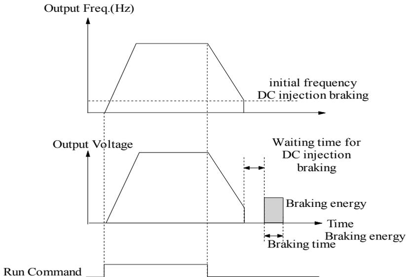
Fig. 5-3-5 DC injection braking
