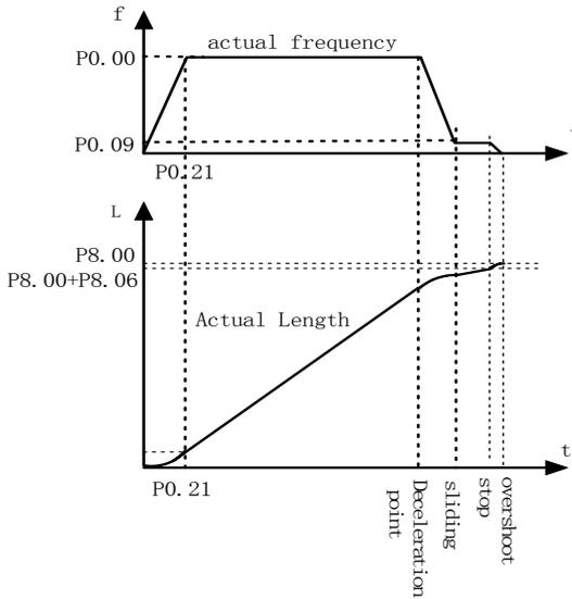
Fig. 5-8-2 Fixed length control diagram 2
