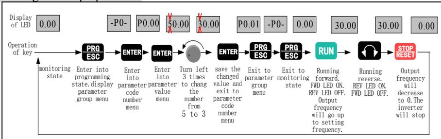
Figure 3-11 Flow chart of running and stop operation
