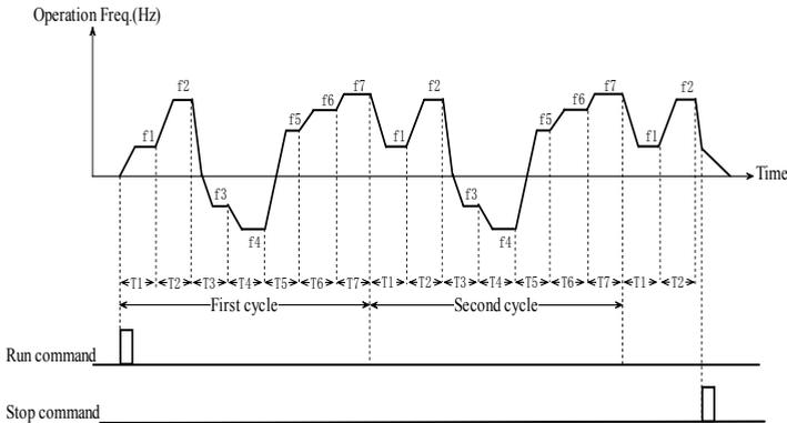
Fig. 5-5-3 Continuous operation of PLC
