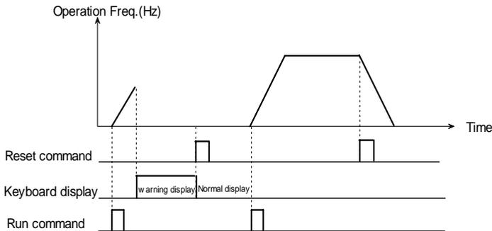
Fig. 5-3-1 Terminal reset
