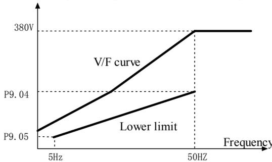
Fig. 5-9-2 Energy saving voltage lower limit
