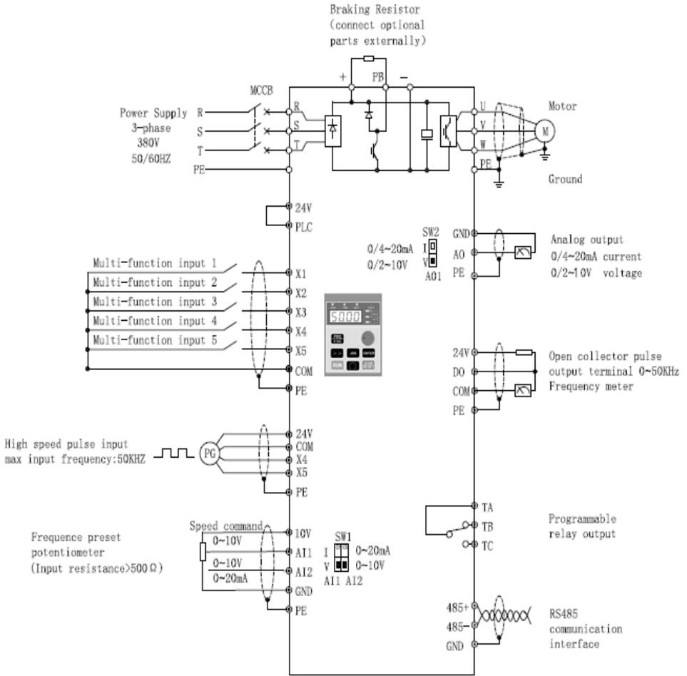
Fig 2-33 3R75GB~3004GB Wiring diagram
