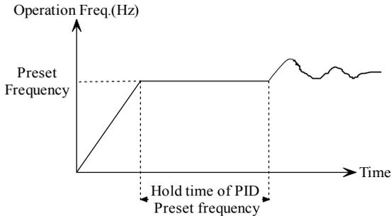
Fig. 5-7-2 PID preset frequency operation
