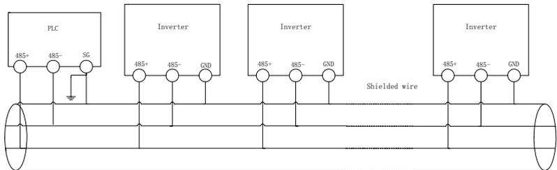
Fig 2-17 Communication between PLC and the Ac drive
