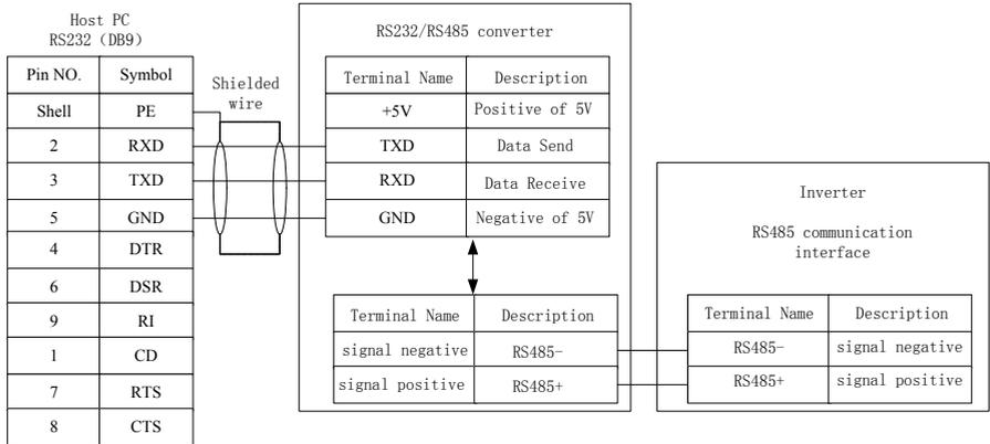
Fig 2-16 Connection between the ac drive and the host PC
