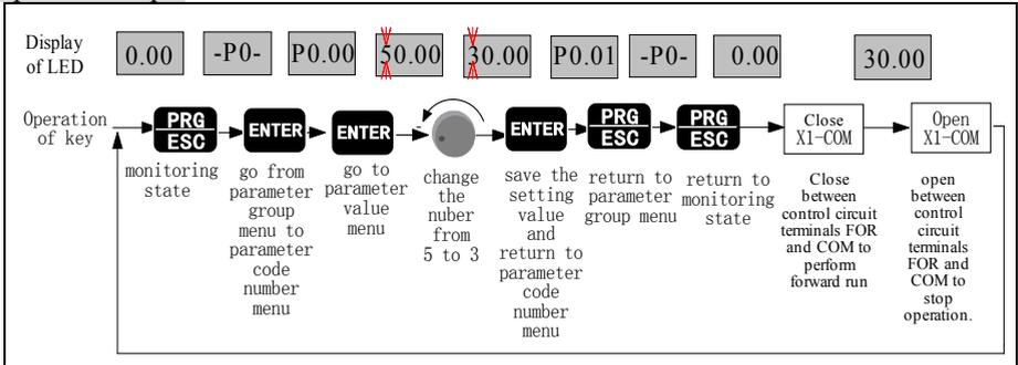
Figure 3-14 Flow chart of running and stop operation by terminal
