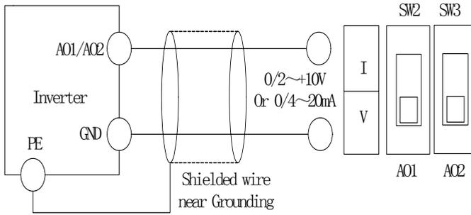
Fig 2-14 S2R4GB~3004GB Analog output terminal wiring diagram
