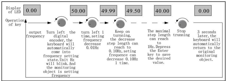
Figure 3-6 Flow chart of frequency setting
