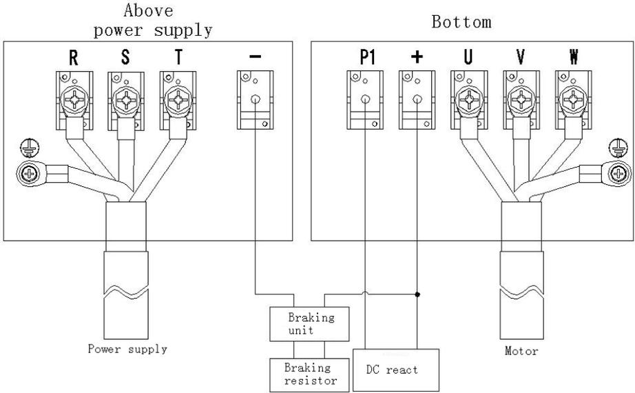
Fig 2-8 3400G~3500G Main Circuit Wiring
