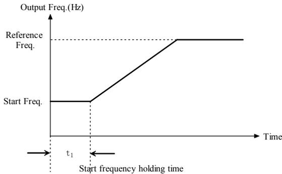
Fig. 5-1-3 Starting frequency and starting time
