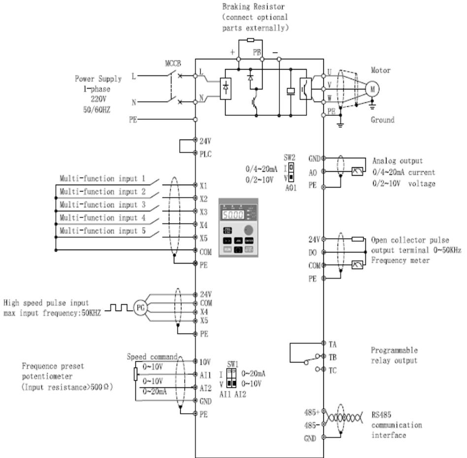
Fig 2-32 S2R4GB~S22R2GB Wiring diagram
