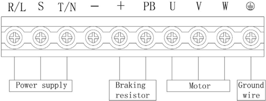
Fig 2-4 3R75GB~3004GB Main Circuit Wiring
