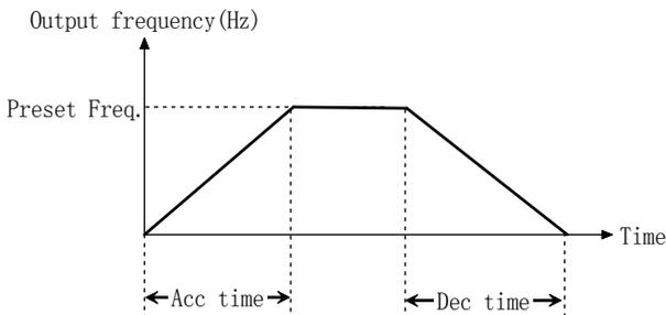
Fig. 5-1-4 Linear acceleration/deceleration
