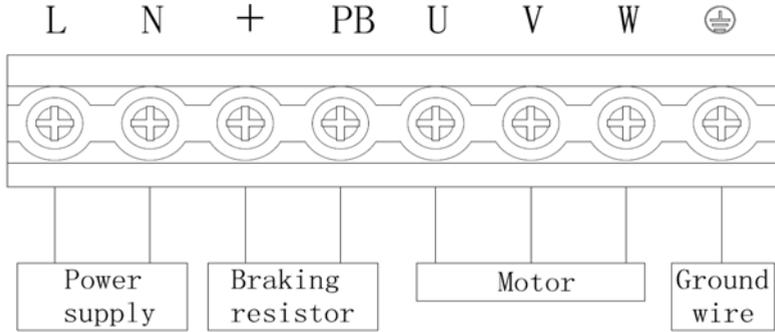
Fig 2-2 S2R4GB~S2R75GB Main Circuit Wiring
