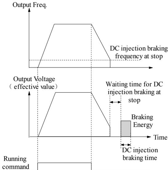
Fig. 5-1-6 DC injection braking
