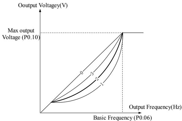
Fig. 5-0-2 Torque-reducing curve
