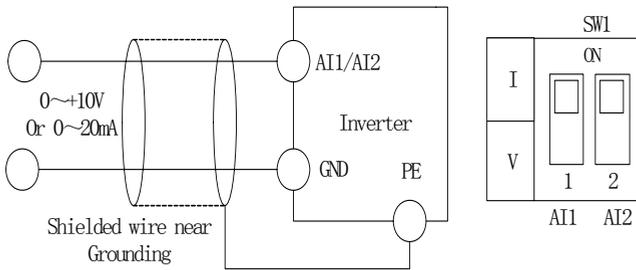
Fig 2-13 Analogy input terminal wiring diagram
