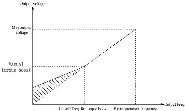
Fig. 5-0-4 Manual torque boost diagram
